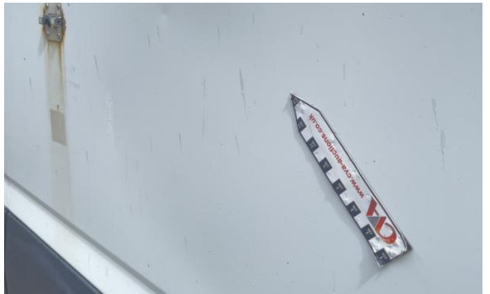
4: Wing osf Dented With Paint Damage
