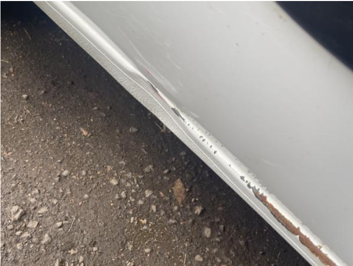
10: Sill ns Dented With Paint Damage
