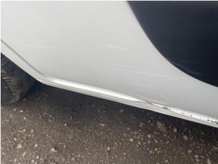
9: Door nsf Dented With Paint Damage
