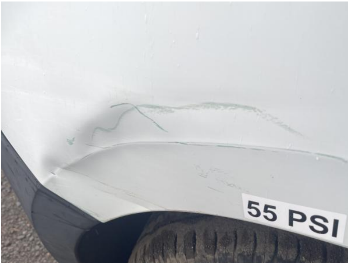
11: Wing nsf Dented With Paint Damage
